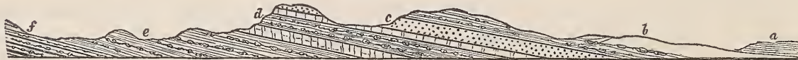
a. Lower Lias. b. Saliferous Marls, &c. c. Red Sandstone and Quartzose Conglomerate. d. Calcareous Conglomerate. e. Lower New Red Sandstone. f. Upper Coal Measures.
