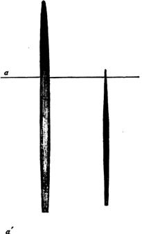
the prism, &c., it was washed with weak gallo-nitrate of silver, the spectrum being shut off by an opake screen. The screen being removed, the luminous image was allowed to act for one minute, and was then again obstructed. The figure (*next page*) shows the chemical image of the spectrum which had not undergone any absorption, and the second that which was obtained when the quinine trough was interposed.
