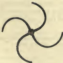
whose motion with the axis or shaft preserves a constant agitation of the semi-fluid mass poured in from the vats. A due portion of quicksilver being added, the two metals will have become united, and sink to the bottom in six or eight hours, leaving the earthy substances still in solu-
