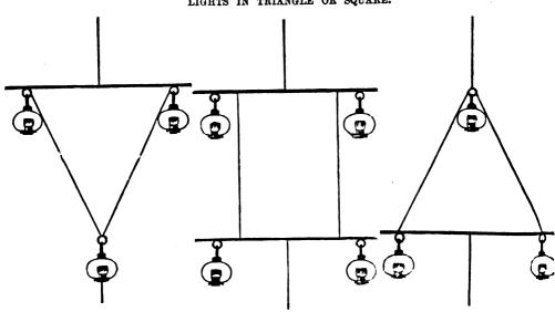
Four lanterns and two yards, each not less than four feet long, will be sufficient — as only one signal will be used at night. These signals may be made with any lanterns, showing either white, or any colour, but dike.
