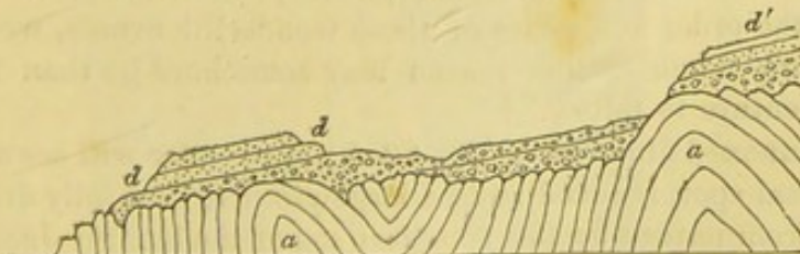
Unconformable junction of old red sandstone and Silurian schist at the Siccar Point, near St. Abb's Head, Berwickshire. See also Frontispiece.
