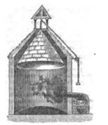
in the iron furnace, and the dense smoke passes into the chamber, which is lined with either sacking or sheepekins. The interior is swept from time to time and sold without any further preparation. The hollow cone of sheet iron inside has a small hole in the top to allow the smoke to escape alowly after it has deposited the greater part of its carbon; by raising and lowering the cone it screpes the sides of the conves or leakher, and detaches the lampblack.—SADDLER, Kendal.
