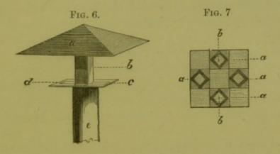
Fig. 6.—a, roof or cover to the stage d; b, pillar which supports the roof a; c, glass slips seven eighths of an inch square; e, socket which fits on to the upper part of a pillar of wood four feet six inches long, and which has its lower extremity fixed into a block of wood which rests on the ground.
