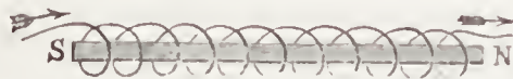
Coil of Electrified Copper Wire turning a Steel Bar into a Magnet.
