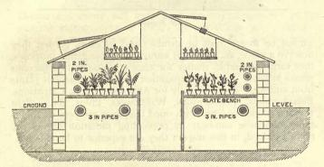
Section of span-roofed Propagating and Hybridising House.
