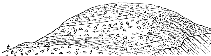
Fig. 32.—Till overlaid with boulder-clay; River Stinchar. r , Rock. t , Till. g , Boulder-clay. x , Fine gravel, &c.
