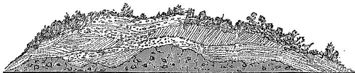
Fig. 37.—Sand and gravel resting on denuded surface of till, railway cutting, near Douglas Mouth Bridge, Lanarkshire.
