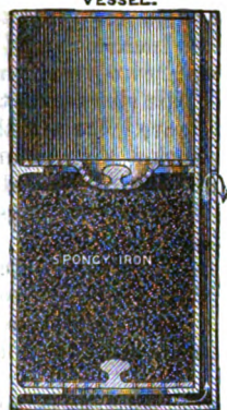
SECTION OF SPONGY IRON VESSEL.
