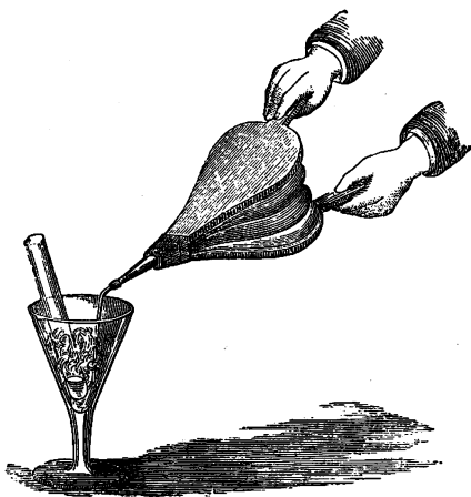
Fig. 184.—FREEZING BY EVAPORATION OF ETHER.
