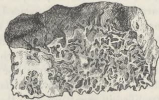
FIG. 84.—A piece of solid limestone bored by Limnoria terebrans , from Ireland.
