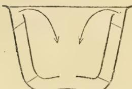
Let this inner boiler have a hole in its bottom, about one third of its diameter, and let its rim be 2 in. below the level of the water to be heated. These arrangements being made, and the heat applied below, a circulation instantly takes place, and continues; the water coming into contact with the heated bottom and sides of the outer boilers, rising rapidly to the surface, and descending through the
