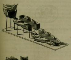
View of a Model shewing the curves generated (experimentally) by the motion of a viscous fluid.
