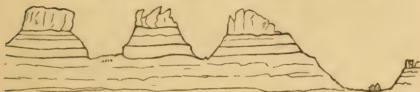
Fig. 1.— Diagram of the Structure of the Mountains of Stratified Rock capped with Basalt, &c. in Southern Africa.
