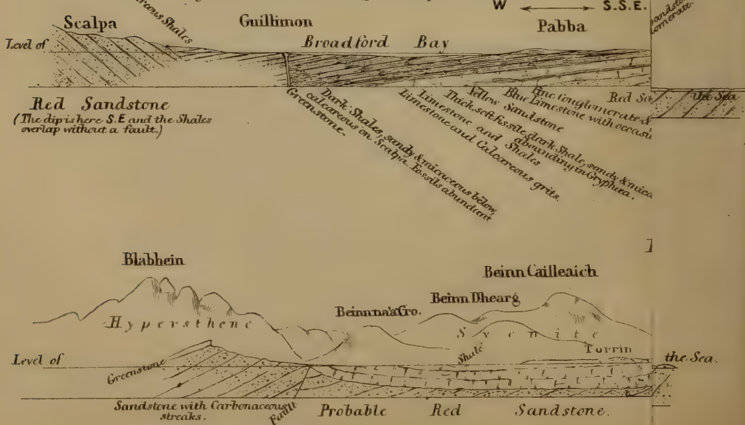
Fig. 2. Section from Scalpa through Guilmion & Pabba to the
