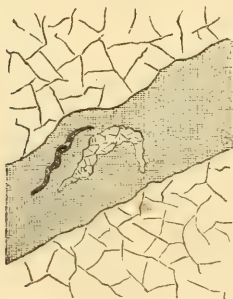
Fig. 2.—Section in the Malvern Tunnel, showing veins of Quartz and Graphite in the band of Chlorite in the Syenite, at 10 m. 792 yds. By Capt. Selwyn.
