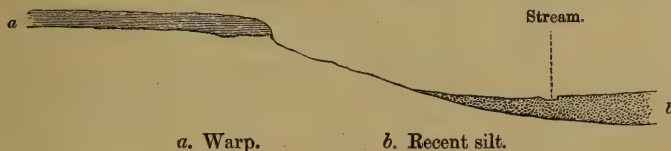
Fig. 11.—Section showing Warp cut off by erosion of a stream.
