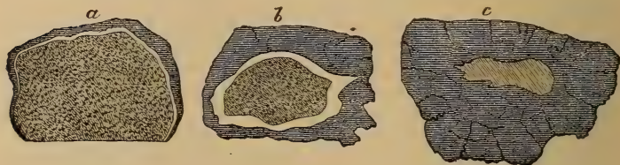
Fig. 63.—“Kernel-roasting” of Copper Ores.
