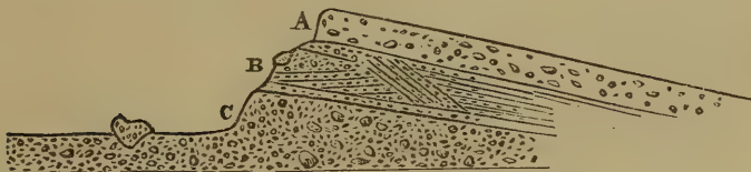
A. Upper Boulder-clay. B. Middle sand, gravel, and "rockery." C. Lower Boulder-clay.
