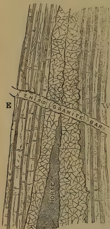
Fig. 6.—Cross section of the Reef, showing third vein of Granite and "Horse."
