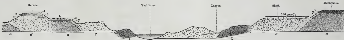
Fig. 2.—Section of the Diamantiferous Deposits on the banks of the Vaal, from Hebron to Diamondia. (Distance about 3000 yards.)
