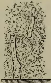
Fig. 2.— Dyke fractured with lateral displacement.
