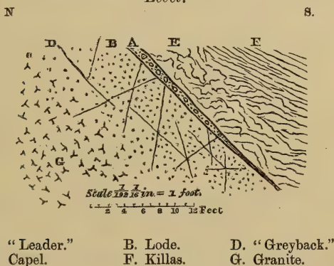
Fig. 1.—Section showing the Lode at Wheal Uny at the 130-fathoms Level.
