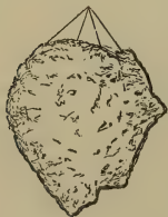
Fig. 1.— Sand-grain with slight deposition of Quartz.
