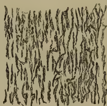
Fig. 6.—Slate, Llanberis, with well-developed cleavage.
