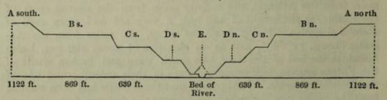
The height of each terrace above the level of the river, is shown by the number under it. Vertical scale  $\frac{1}{20}$  of inch to a 100 feet; but terrace E being only twenty feet above the river, has necessarily been raised. The horizontal distances much contracted; the distance from the edge of A n. to A s. being on an average from seven to ten miles.
