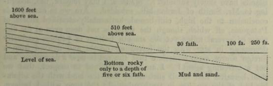
Vertical and horizontal scale, two inches to a nautical mile. The point marked 1600 feet is at the foot of High Knoll; point marked 510 feet is on the edge of Ladder Hill. The strata consist of basaltic streams.
