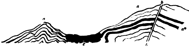
a. Contorted culm strata with stone coal. b. Fault. c. Slash of finely triturated culm between violently contorted strata, and probably upon a great line of fracture.
