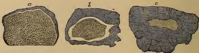
Fig. 63.—“Kernel-roasting” of Copper Ores.
