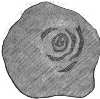
No. 4. Section 6 feet below where a large branch had been taken off, disappears about 9 feet down ; all above where the branch springs from quite sound ; all contained within the irregular curved lines is rotten wood.
