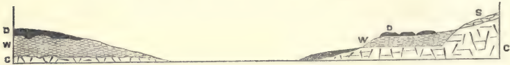
Diagram CCI. Section across the Vale of Kennet. C. Chalk. W. Woolwich beds. S. Sarsen stone. D. Drift.
