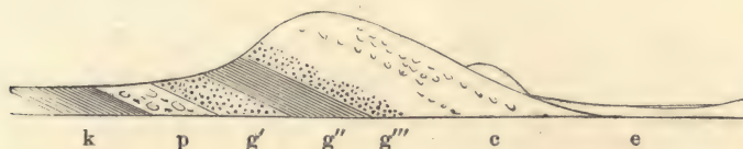
Diagram IX. k. Kimmeridge clay. p. Portland rock. g'. Lower green-sand. g''. Gault. g'''. Upper green-sand. c. Chalk. e. Eocene strata.
