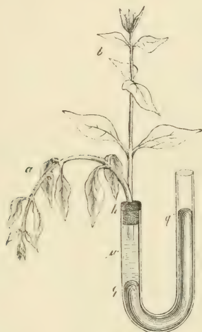
FIG. 439.—Apparatus for showing the revival of withered shoots by forcing water into them. The U-shaped glass tube is first filled with water, and the perforated stopper of caoutchouc h in which the stalk of the plant is inserted, is then fixed in. When the shoot is withered, as represented by a , mercury is poured into the other arm of the tube, so as to stand at q' some 8 or 10 cm. above q , and the shoot then revives, as represented by b , even when the level q becomes subsequently higher than q' .
