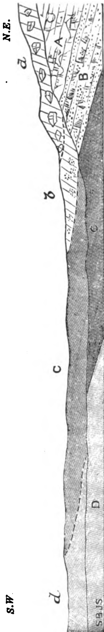
FIG. 21.—Diagram Section showing the site and character of the Boulder Clay, etc., just north of the Fens.
