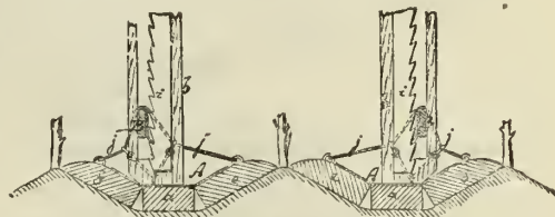
FIG. 32.—HELM BRUSHING-MACHINE: transverse section of lower part.
