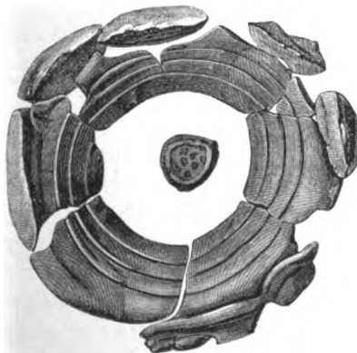
Fig. 85.—Ex.—Lead Bullet after Projection in Water, drawn from Object, Full Size.
