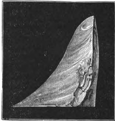
Fig. 76.—Ex. Conoidal Splinter of Glass. Drawn by Mr. Collings.
