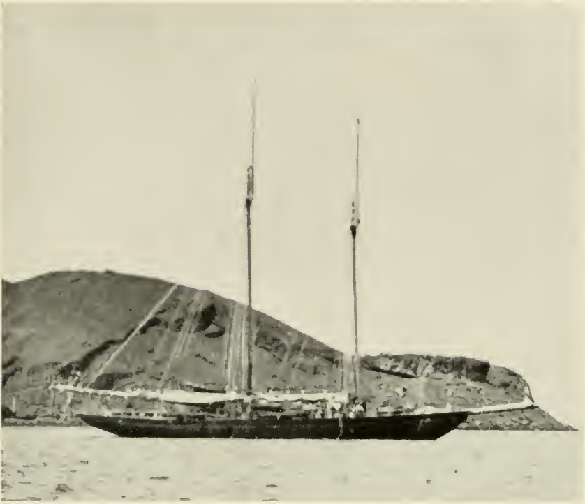
Fig. 26. Templeton Crocker's yacht Zaca , 118 feet over all, was a strongly constructed two-masted schooner and a deep-sea vessel. Her cruise to the Galápagos was a noteworthy one, both from the standpoint of surveying and that of natural history.
