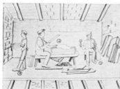
FIG. 8. Slate quarry workers. (1) Splitting slabs, (2) measuring and trimming slabs, and (3) apprentice. Sketched by the Welsh artist, historian, and linguist, Mr. Elfed Thomas, of Nant Peris.
